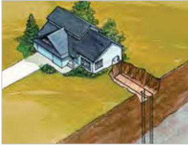
At Sun Rivers, Corix Utilities installs and manages vertical ground-source heat loops as community infrastructure. Residents are billed a monthly ground loop access fee as part of their utilities, and save on monthly energy bills. Source: WaterFurnace International
