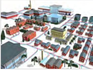
District energy for a community: Red lines: heating supply; blue lines: cool water return. For a small neighbourhood system, heat may be supplied by solar hot water panels, ground-source heat pumps, a small biomass plant and/or heat recovery from a diesel generator (e.g. in a remote community). Source: Vital Energi Utilities Ltd
