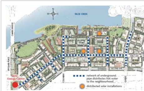
Extent of the Neighbourhood Energy Utility in Vancouver's South East False Creek. The district energy service is owned and operated by the City of Vancouver. Source: City of Vancouver
