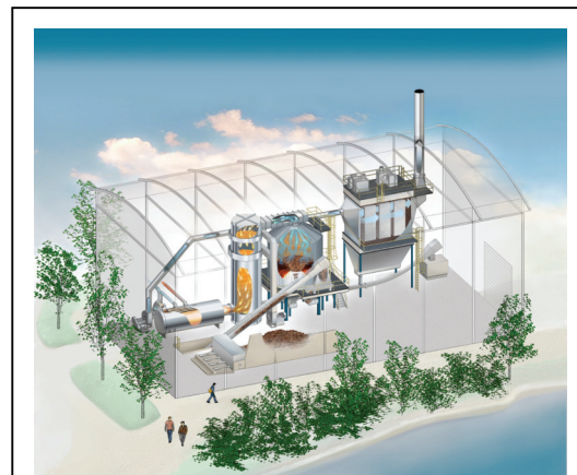
Illustration of the Nexterra district heating system for the Dockside Green residential development on Victoria's inner harbour.
